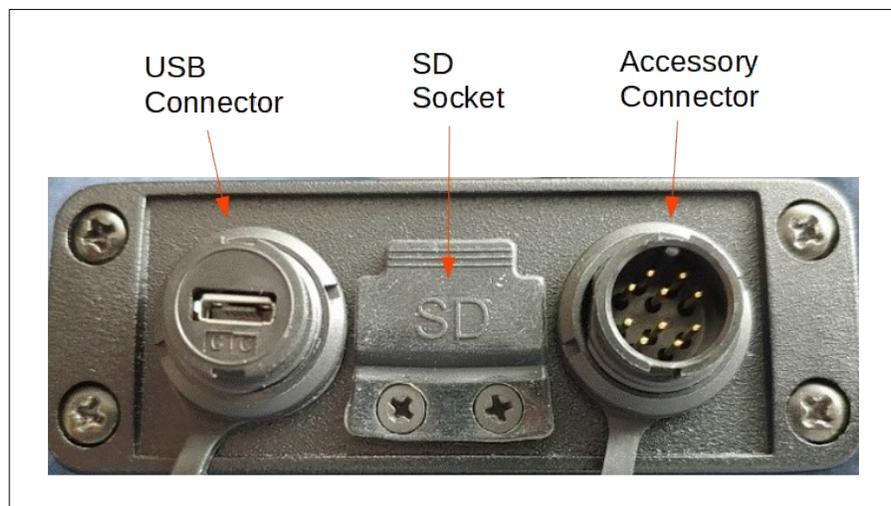
The USB connector can be used for charging the receiver. The receiver is provided with a USB cord for this purpose which can be used with any 2.5A 5V USB charge adaptor commonly used with cell phones. The receiver will charge fastest with the power turned off. Currently the USB connector is not available for data connections.
