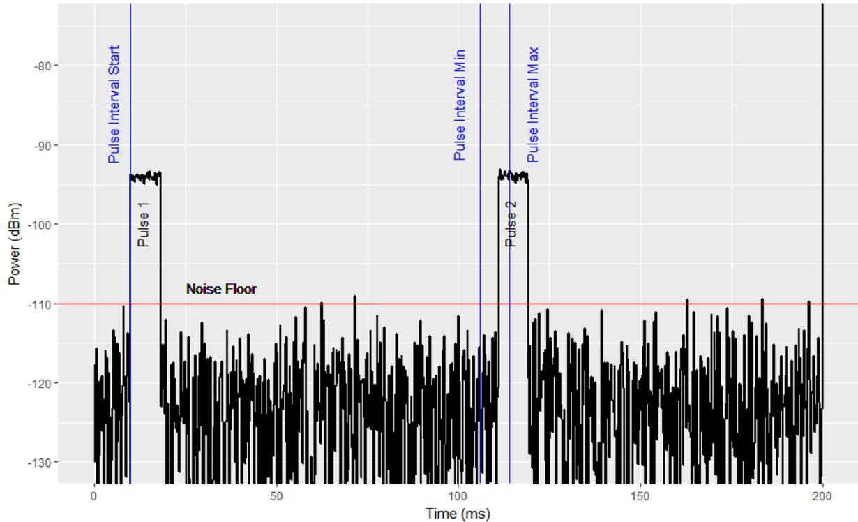
Figure 6: How pulse interval is calculated
