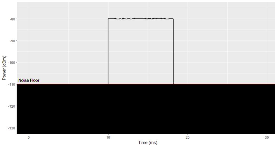
Figure 2: How a receiver sees the incoming signal after taking into account the noise floor, or squelch level
