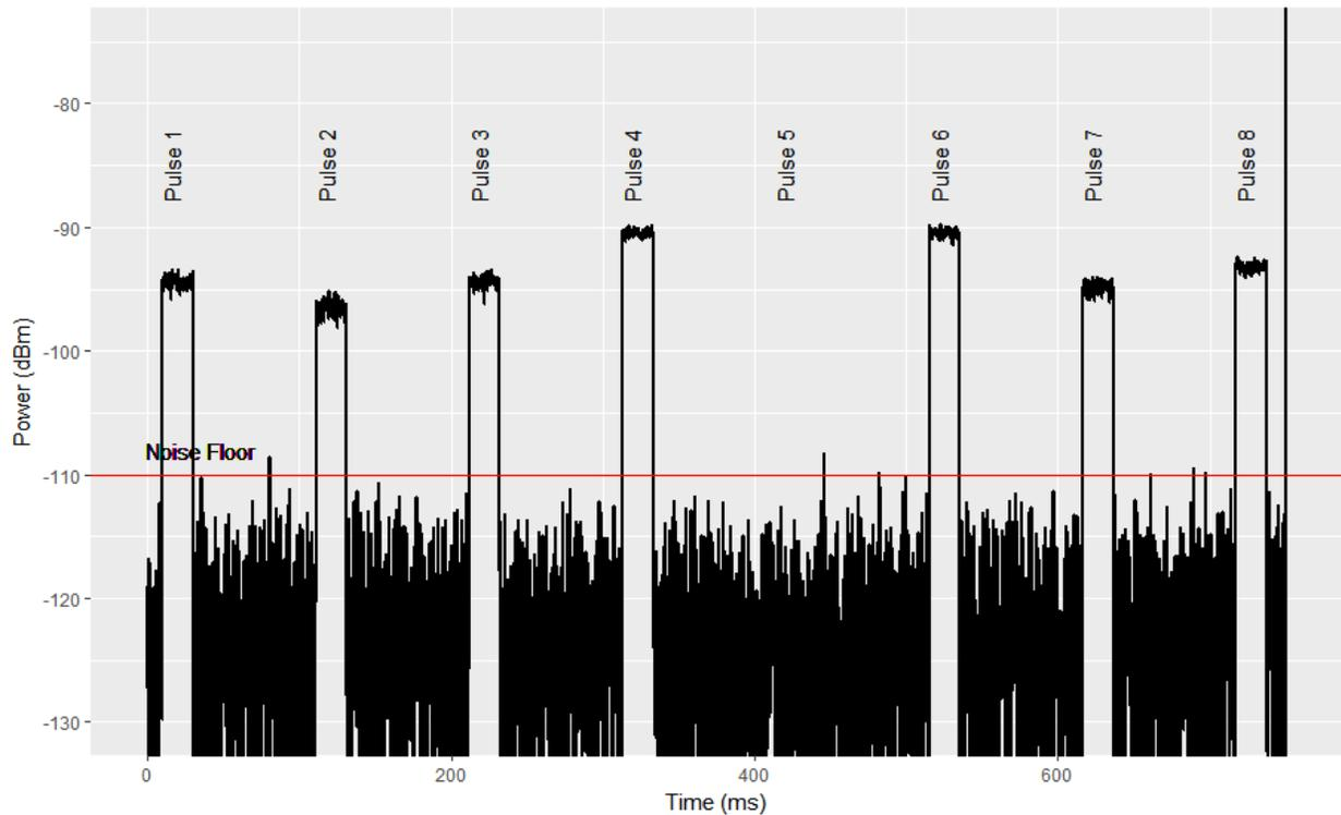
Figure 7: Beeper transmitter emitting a 20ms pulse every 100ms starting at 10ms
