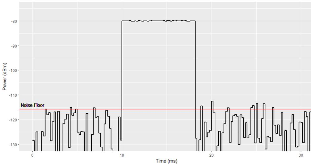
Figure 1: Beeper pulse superimposed on the background noise. A red line is drawn across at roughly 5dBm above the average noise level.
