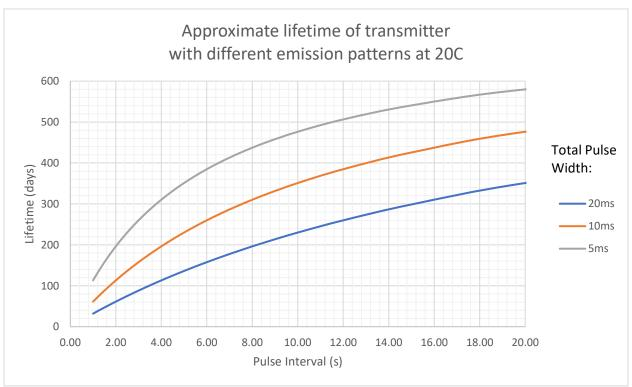
Note: Lifetime can be increased significantly (more than shown above) with the use of programming features such as date/time control.
